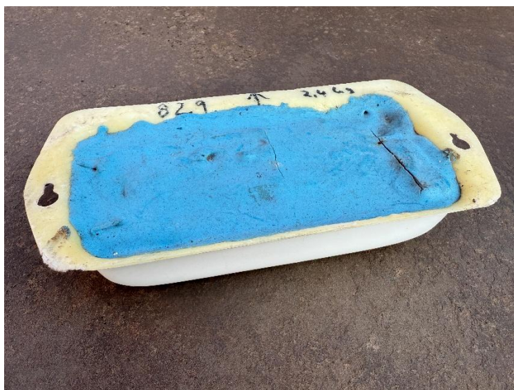
Charger 2.4kg corrector weight showing slotted holes for fixing to underside of deck
